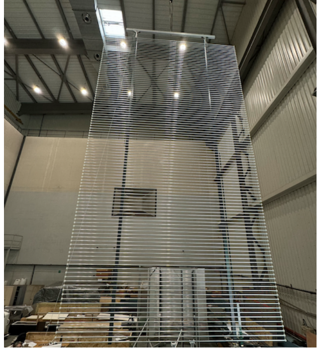
Figure 2: Field cage construction for Mock-Up at B. 185, CERN.
